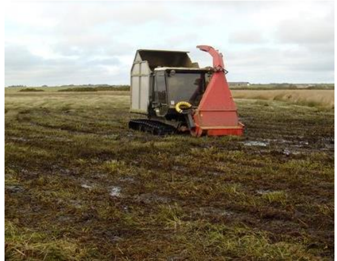
Figure 2. Specialised mower cutting Moss Town Fen. The tracked wheels reduced ground pressure enabling the contractor to cut areas of the fen that would be too boggy for conventional machinery.
