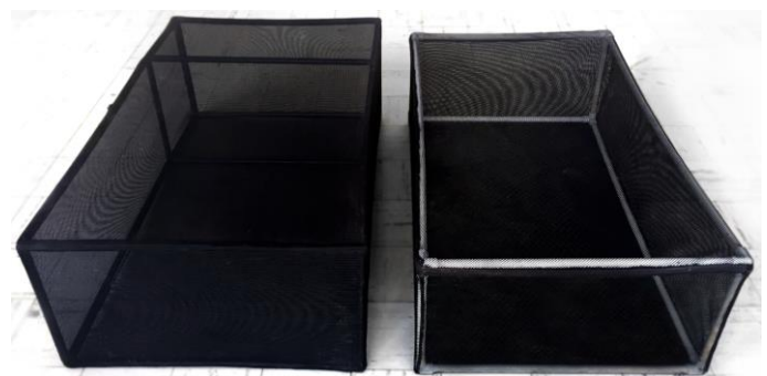
Figure 4. Aquatic mesh cages where captive-reared crawfish frog Lithobates areolatus tadpoles completed development in 2014–2015. A 380 L Reptarium® is on the left, a 285 L custom cage on the right.
