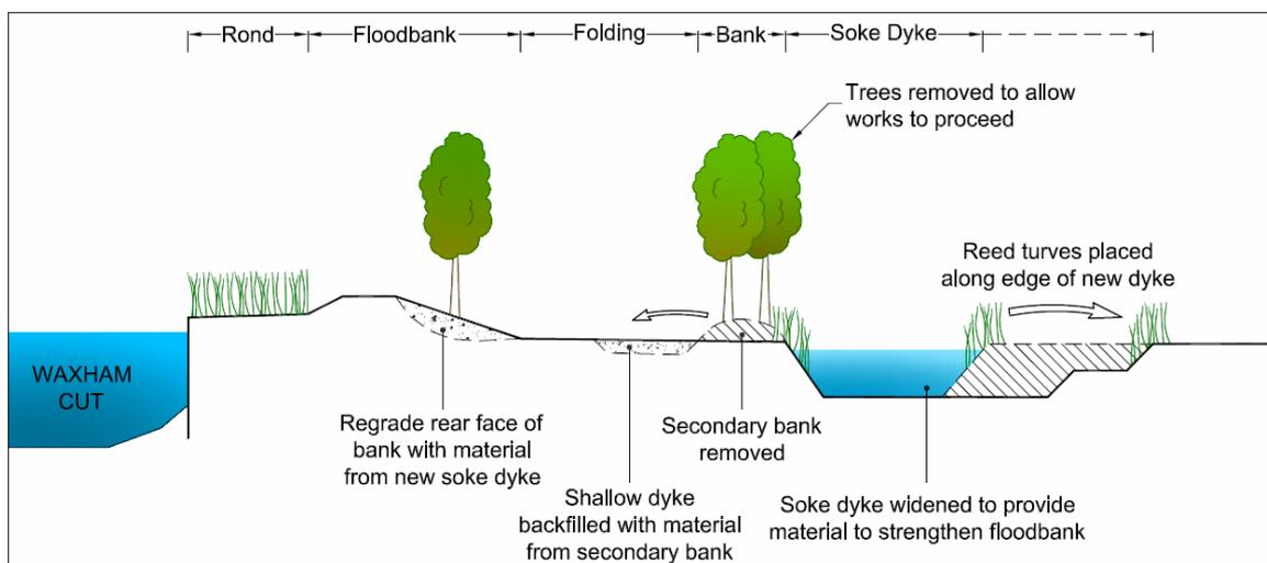
Figure 2. Proposed flood defence works – typical cross section
