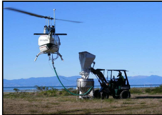
Figure 2. Helicopter with bait spreading bucket being filled by loader.
