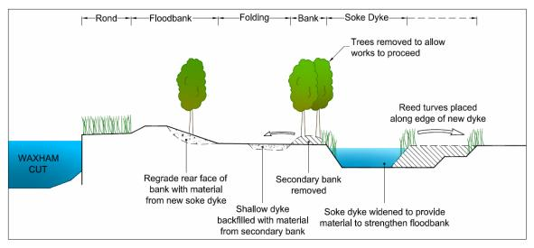
Figure 2. Proposed flood defence works - typical cross section
