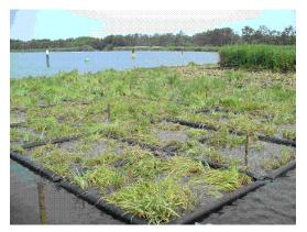
Figure 1. The floating island showing the plastic floats supported by metal grids and recently planted vegetation.
